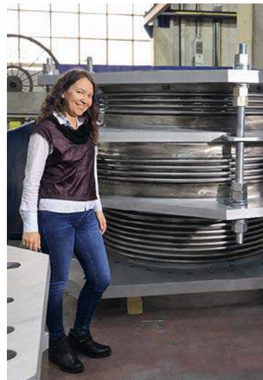
Bediha on site with an expansion joint.
