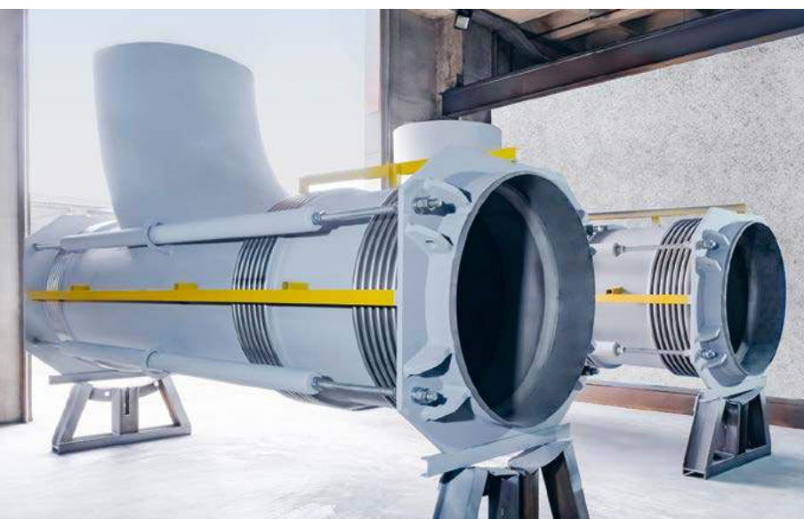
Custom expansion joints being prepared for Dradenau.
