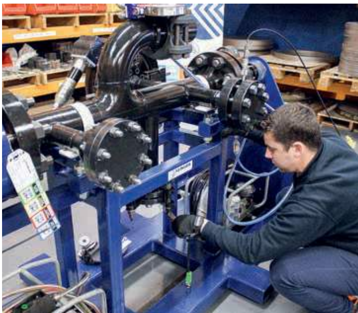
Scott Whelan bolts a flange.
